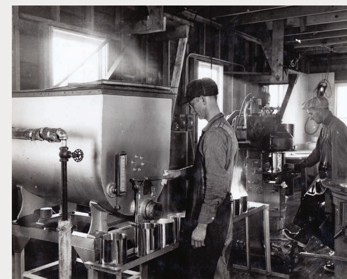
The recipe for canning carp was 150 gallons of fish and 60 pounds of flour, heated to 180 degrees. The first cannery was at Nevin Fish Hatchery in Madison.
