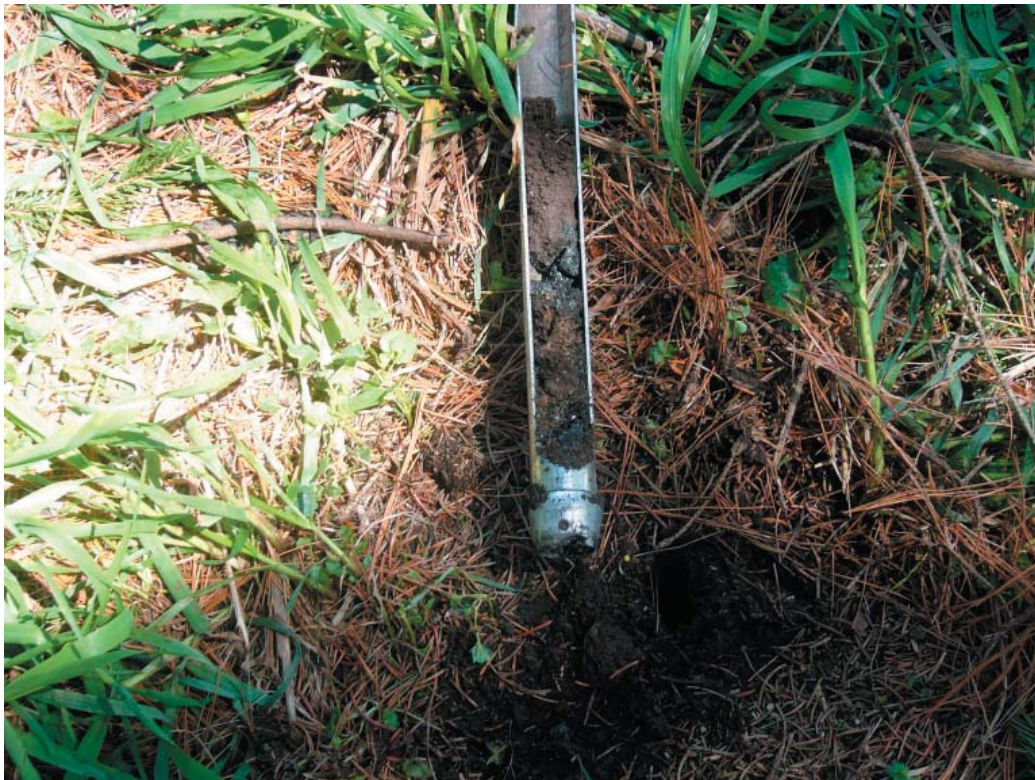
Soil core of cinder pile south of Dormitory for Help.
