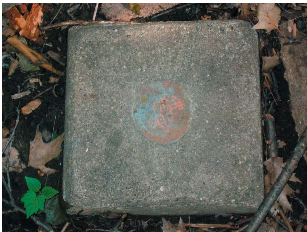
USGS benchmark located in woods on Lake View Hill County Park property.
