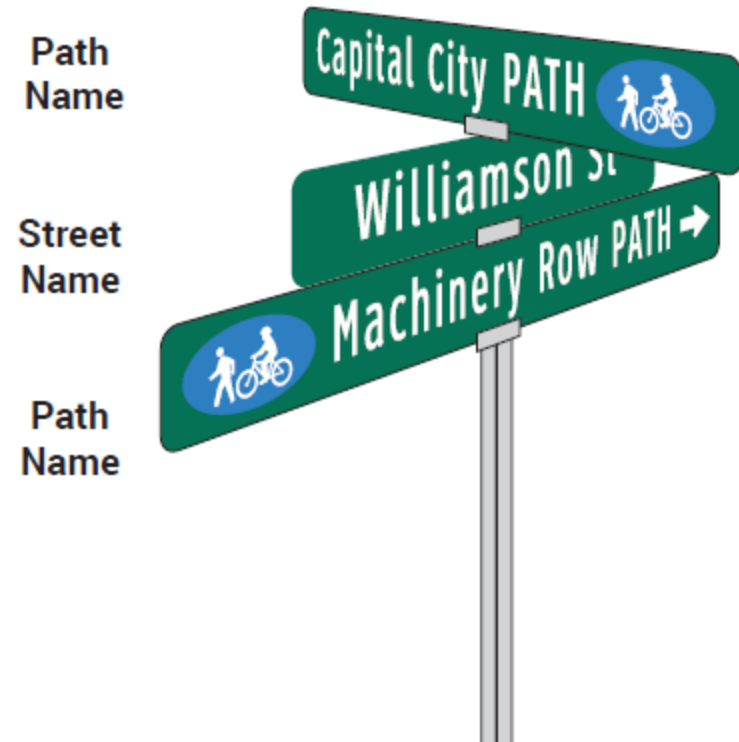
Double-sided street name assembly with multiple path names
